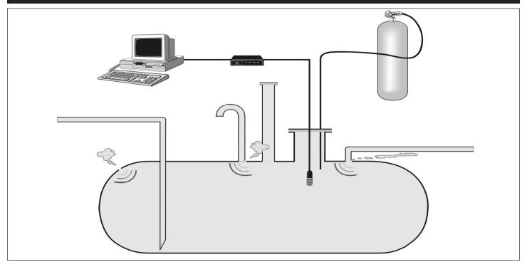
The integrity of a storage tank can be verified and in a short period of time with the sonic leak detection test. This technique has been third party performance evaluated and generates reliable leak detection test results in a cost-effective manner.
